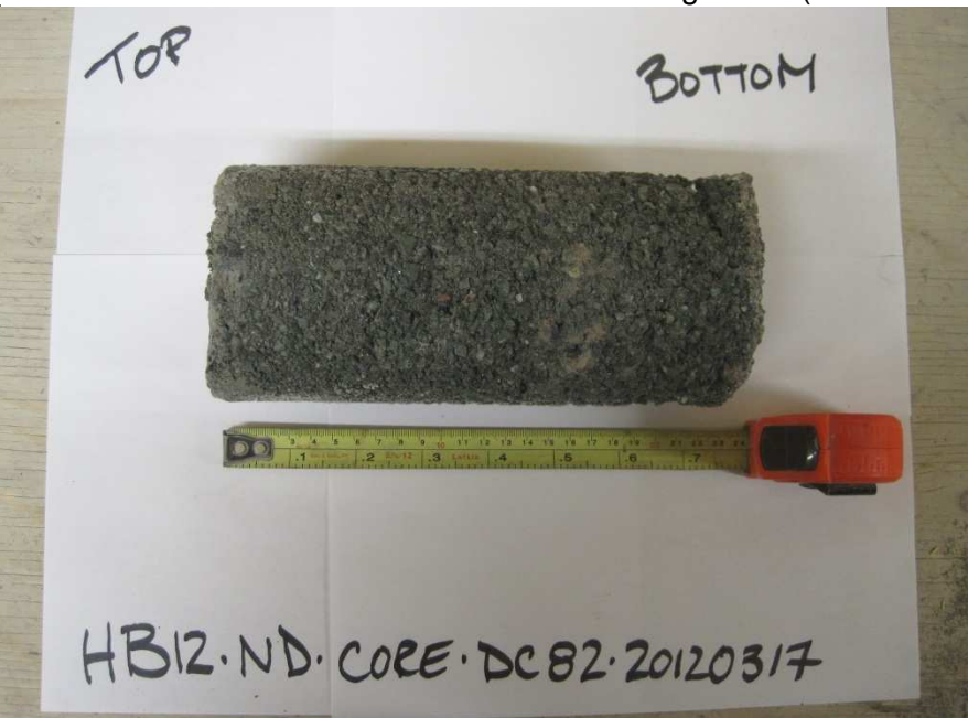
Photo 18: Drilled Core 82. Taken from ~ 1+20 CL
